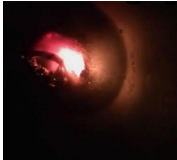
A C.Joule Effect. Inc, test: joule effect, glowing connection. No arc, temperature to over 1148°F.
